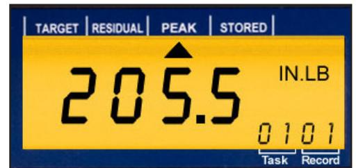
When the torque specification is achieved, the light turns bright green. All the operator needs to do is stop applying force - "Green is Good!"
