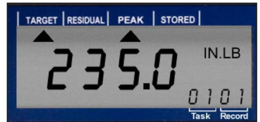
As the operator begins applying torque to the first fastener, the display changes to provide current information on the status of the torque application. The current torque shows as it is applied, and when the operator gets close to the torque specification, an LED emits a bright yellow-orange light that backlights the display and appears in a prominent lens on the back of the wrench. Warning - you're getting close!
